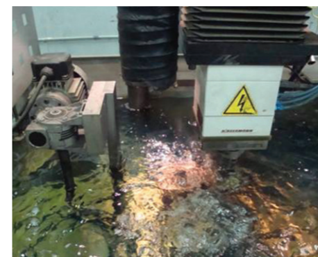
The Electrical Discharge Machining (EDM) process is a critical step in precision re-dressing of CNC tooling.
