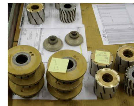
Worn CNC tooling is logged in and prepared for re-dressing.
