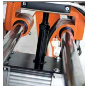
Linear bearings with chrome plated steel bars.
