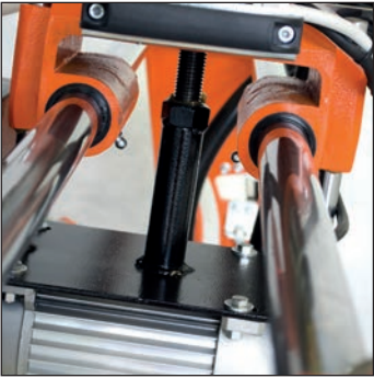
Linear bearings with chrome plated steel bars.
